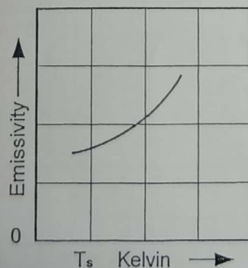
Fig.3 Variation of Emissivity with surface temperature
